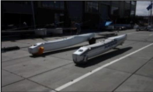
1. Place the starboard and port hull next to each other and make sure that the hulls are facing the same way
